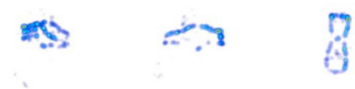
Figure 4: L_p regularized least-square reconstructions of a civilian vehicle from GOTCHA dataset (3-D, Side and Top Views, p = 1 and \lambda = 10 ).
